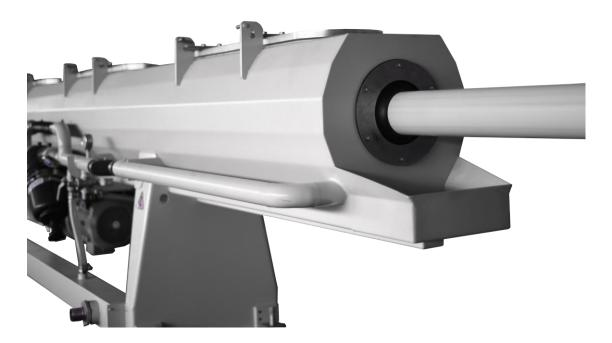
Pipe extrusion is a manufacturing process in which molten plastic is pressed through a nozzle to form a continuous pipe. The nozzle is shaped to the desired cross-section of the pipe, and the molten plastic is cooled and solidified as it passes through the nozzle. Pipe extrusion can be used to produce a wide range of pipe sizes and shapes, from small irrigation pipes to large sewer pipes.
